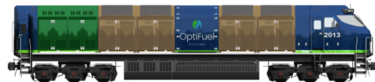
80' 5000 hp Line Haul Locomotive, AC Traction
