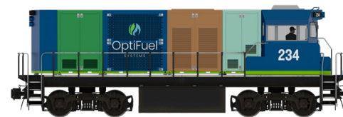
52' 1000-1800 hp Switcher Locomotive, DC Traction
