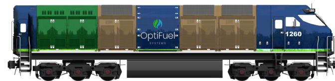
72' 4600 hp Line Haul Locomotive, AC Traction
