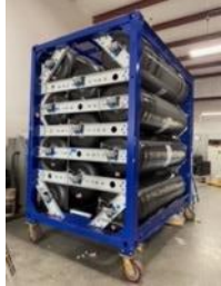
H 2 On-deck Storage QD Module
